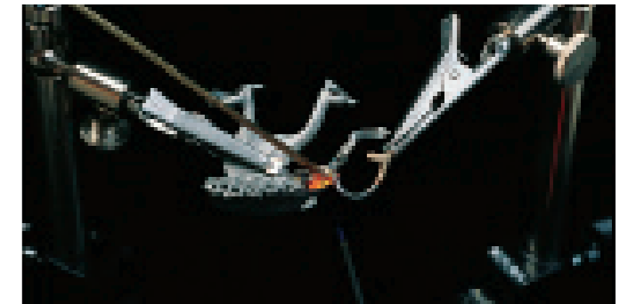
Soldering of a prefabricated gold clasp
