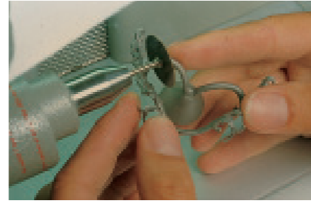
Disconnecting the sprues
