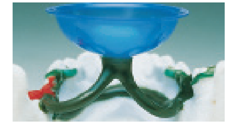
Sprue attachments in lower jaw, casting from above
