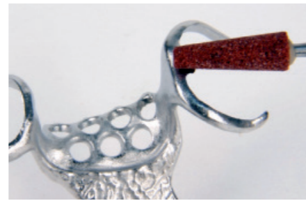
Finishing with corundum or fine grinding stones
