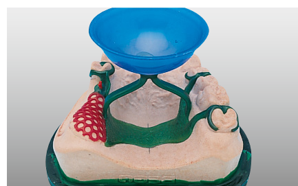
Sprue attachments in upper jaw, casting from above
