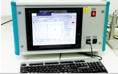
Quality control with state-of-the-art equipment: the dilatometer determines the thermal expansion of the BEGO investment materials
