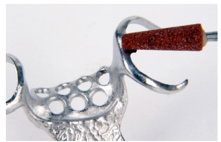
Finishing with corundum or fine grinding stones
